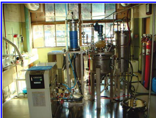
Figure 5. Continuous pilot plant for the degradation of PCBs under mild conditions.
